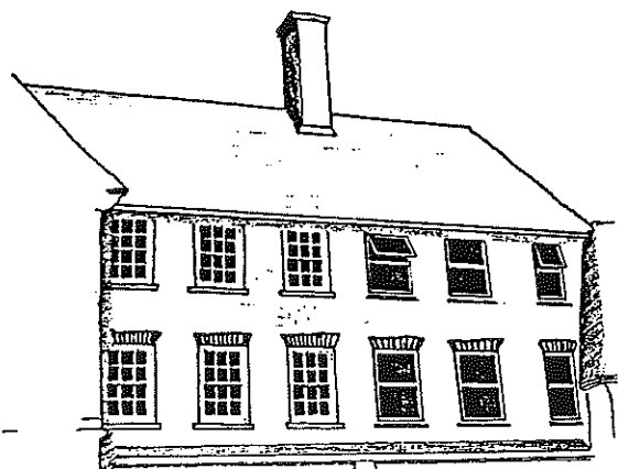
Example of Undesirable replacement windows
